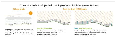
Along with the European-based Enertis Applus+ IE report (June 2023) that found **1-2 percent energy gains** from TrueCapture's Split Boost Mode for half-cell modules, the new ICF analysis adds to a growing collection of independent engineering studies proving TrueCapture's system control capabilities.
